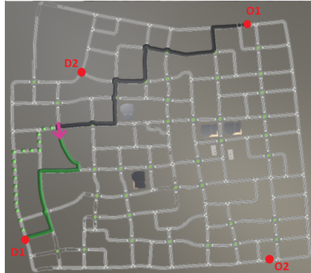
Figure 1: Map of the city. Red dots: Origin and destination pairs, O_1 , D_1 , O_2 , D_2 . Magenta arrow: AV's current location and orientation. Black solid line: path has already passed. Green solid line: planned optimal path to the destination. Dotted light green line: previous planned optimal path to the destination before error occurs.
